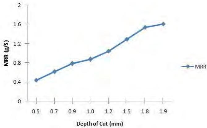
Figure 2: Effect of Depth of Cut on MRR
