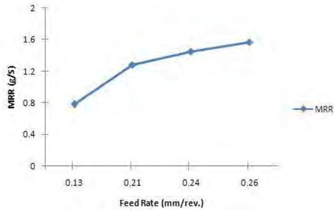
Figure 3: Effect of Feed Rate on MRR
