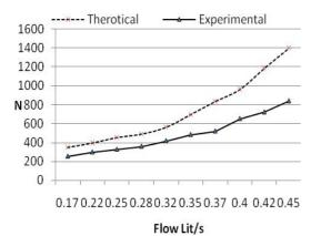
Fig. 5b : A plot of Flow v/s Speed for 6 smooth discs and 0.5mm spacing
