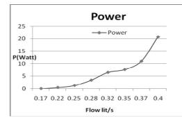
Fig.7 : A plot of flow v/s Power at various flow rates for six discs and 05mm spacing.
