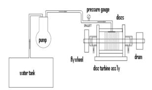
Fig. 4 : Experimental Set up.
