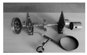
Fig. 2 : Parts of Multiple disc Turbine.
