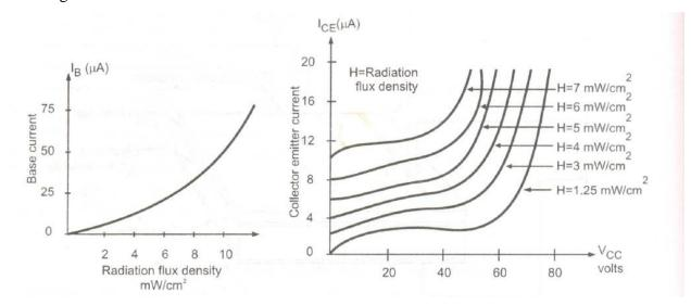
The fig .shows the graph of base current against  $\cdot$  the radiation flux density measured in mW/ cm2. The Fig. (b) shows the collector characteristics of a phototransistor. As light intensity increases, the base current increases exponentially.
