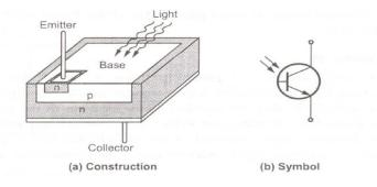
To generate more base current proportional to the light, larger physical area of the base is exposed to the light.
