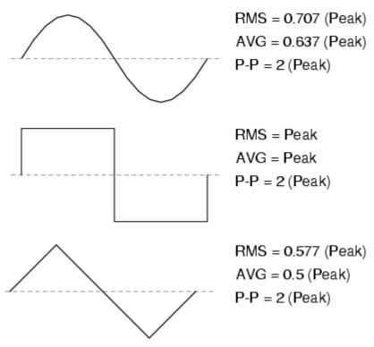
Conversion factors for common waveforms.
