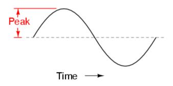
Peak voltage of a waveform.
