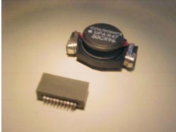
Figure 2. An integrated inductive component (left) and a drum core (right) are shown.
