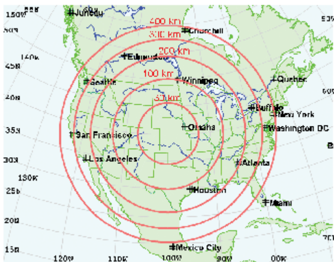
Figure 4. Indication of the area exposed to E1 HEMP from a high-altitude burst over the central United States for various burst altitudes given in km.
