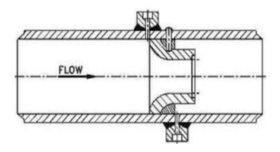
As compared to the orifice plate, flow nozzle is better option as no possibility of solid particles or bubbles of gas sticking in the flow restriction. The flow across nozzle is as shown in the figure below.
