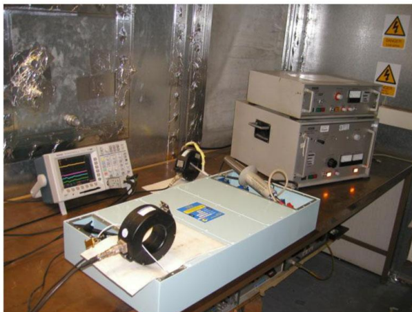
Figure 5: MPE Laboratory Pulse Test Set-Up
