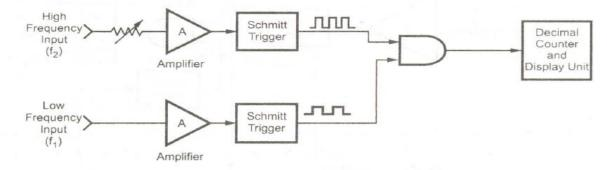
In this mode, the low frequency signal is used as gating signal, while the pulses are counted for the high frequency signal. Hence it is clear that the low frequency represents the time base. The number of pulses corresponding to the high frequency signal f2 are counted during the period of the low frequency signal f1, by the decade counters and displayed by the display unit.
