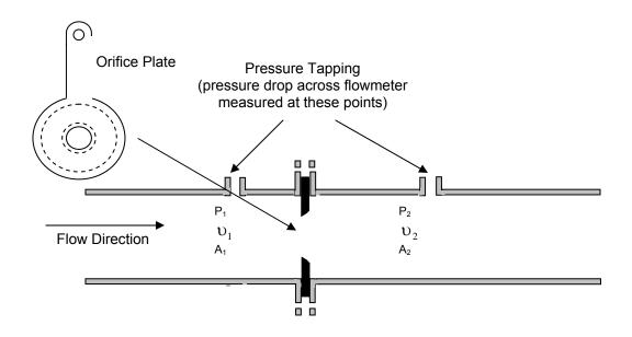
Figure 1: A Concentric Sharp Edged Orifice Plate Flowmeter
