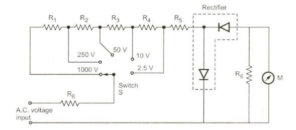
The rectifier used in the circuit rectifies a.c. voltage into d.c. voltage for measurement of a.c. voltage before current passes through the meter. The other diode is used for the protection purpose.
