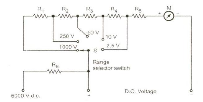
For getting different ranges of voltages, different series resistances are connected in series which can be put in the circuit with the range selector switch. We can get different ranges to measure the d.c. voltages by selecting the proper resistance in series with the basic meter.
