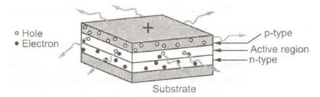
One of the methods used for the LED construction is to deposite three semiconductor layers on the substrate as shown in the Fig In between p type and n type, there exists an active region. LED Driver Circuit:
