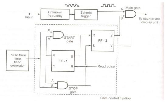
The output of unknown frequency is applied to the Schmitt trigger which produces positive pulse at the output. These are **counted pulses** present at A of the t11<lingate. The time base
