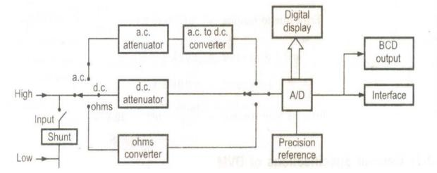
The current is converted to voltage by passing it through low shunt resistance. The a.c. quantities are *converted* to d.c. by employing various rectifier and filtering circuits. While for the resistance measurements the meter consists of a precision low current source that is applied across the unknown resistance while gives d.c. voltage. All the quantities are digitized using analog to digital converter and displayed in the digital form on the display.
