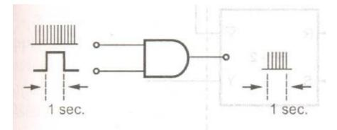
The signal waveform whose frequency is to be measured is converted into tngger pulses and applied continuously to one terminal of an AND gate. To the other terminal of the gate, a pulse of 1 sec is applied as shown in the Fig. The number of pulses counted at the output terminal during period of 1 sec indicates the frequency.
