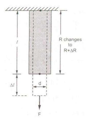
$$\frac{dR}{d\sigma} = \frac{d\left(\frac{\rho l}{A}\right)}{d\sigma} = \frac{\rho}{A} \frac{\partial l}{\partial \sigma} - \frac{\rho l}{A^2} \frac{\partial A}{\partial \sigma} + \frac{l}{A} \frac{\partial \rho}{\partial \sigma}$$
