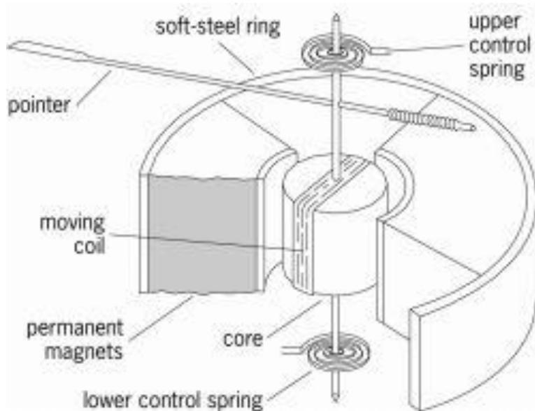
When an electric current is passed through a coil placed in a magnetic field, it experiences a force. This force causes a torque in the coil that is fixed to a spindle. The spindle can rotate in fixed bearings.
