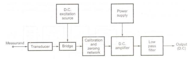
The resistance transducers are commonly used for the d.c. systems. The resistance transducers like strain gauge forms one or more arms of a wheatstone bridge circuit. A separate d.c. supply is required for the bridge. The bridge is balanced using potentiometer and can be calibrated for unbalanced conditions. This is the function of Cdlibration and zeroing network. Then there is d.c. amplifier which also reqUIres i..l separate d.c. supply.
