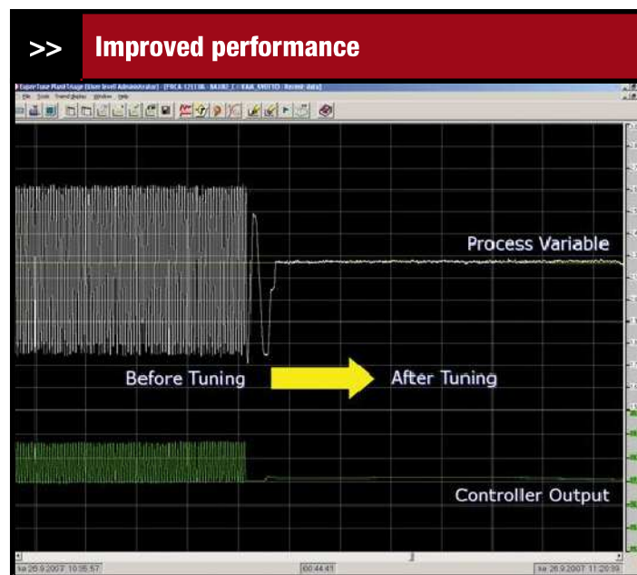
Figure 3. Effective tuning provided close-to-optimal control of process variable.
