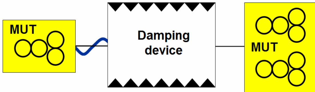
Figure 6: pulsations should be isolated by damping device
