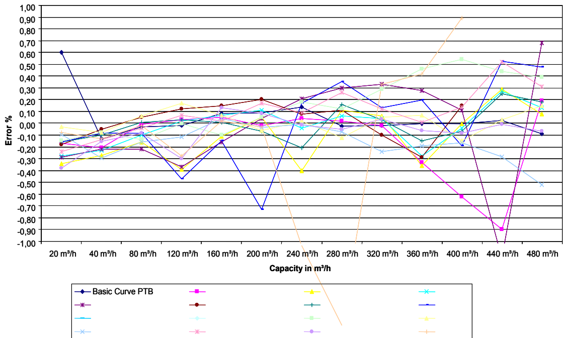
Figure 4: Pulsation effect on different types of test benches
