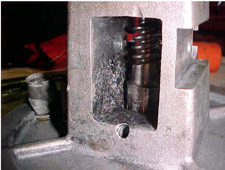
Figure 1 :Damaged Ball Bearings of a G650 Turbine Gas Meter caused by a Shock during Transportation.
