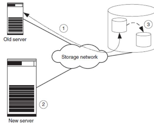
**Figure 1.4** The old server is connected to a storage device via a storage network (1). The new server is assembled and connected to the storage network (2). To generate test data the production data is copied within the storage device (3).
