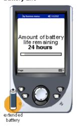
Most PDAs are now provided with an integrated rechargeable battery which recharges while connected to a base station or power adaptor. The most common type of rechargeable battery may be Lithium Ion (Li-Ion), and a general gauge of a battery's capacity is provided in terms of mAh (milliAmp hours). Although real-world performance will vary among devices and how they are used, a battery with a higher mAh value will be able to hold a greater charge and last longer between charges.
