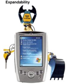
PDAs generally come with a base amount of memory on board for storing data and applications, but they can be filled up quite quickly. Most of these devices now include slots that will accept some sort of flash memory to increase their capacity (Click here for Tech Tips on Flash Memory):Part I and Part II. Typical formats supported by PDAs include: Compact Flash, SD, MMC, or Memory Stick.
