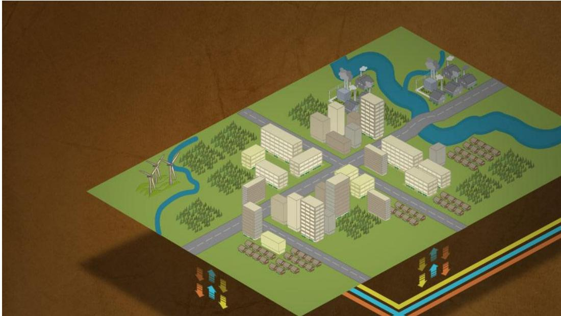
A groundbreaking project is currently being implemented on the Hönggerberg Campus of renowned Swiss Federal Technical Institute, [ETH Zurich](#). In the future, waste heat from buildings on the Science City Campus will be stored in the earth during the summer through 800 ground probes.
