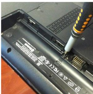
1. Remove the bottom keyboard screw. Flip the laptop over, and look for a screw hole that has a picture of a keyboard next to it and remove these screws. Note that some keyboards don't have a bottom screw.
