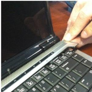
3. If the trim piece between the keyboard and screen is secured to the bottom assembly with clips, then using a credit card or similar (nondestructive) tool you can work your way along the edge in the seam between the trim piece and the laptop and carefully pop the piece up. In my experience, you don't want to use a screw driver, since this may mar the plastic. If some wires are attached to the trim piece simply unplug it and set the trim piece aside.
