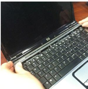
4. Remove the top screws that hold the keyboard in place. In the area where you removed the top trim piece, you should now see three or four screws on the top portion of the keyboard securing it into place – take these out and then carefully lift the keyboard up and back towards the screen and then flip it forward upside down on the palm rest.
