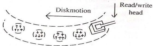
Fig. 14 Individual bits encoded on a disk track.
