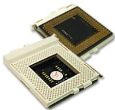
Intel's latest offering for their Pentium 4 and Celeron processors, LGA 775, doesn't have pins at all and basically swaps the pins to the motherboard for the socket. Perhaps this design move puts the burden of bent pin warranty
