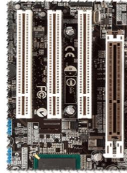
may typically feature four to five PCI slots, and although they could be used for secondary display graphics cards, more common applications include sound cards, network cards, RAID controllers, TV tuners, modems, and USB/Firewire controllers. Considering that many of these items are now included onboard, having multiple PCI slots isn't quite as important as it used to be.
