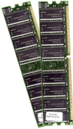
having 240 pins prevents them from being interchangeable. Going forward, users will have to decide whether they want to jump on the new technology bandwagon when selecting a motherboard, or to try to continue using their existing DDR for as long as possible.
