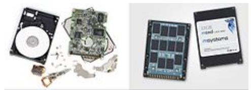
The disassembled components of a hard disk drive (left) and of the PCB and components of a solid-state drive (right)
