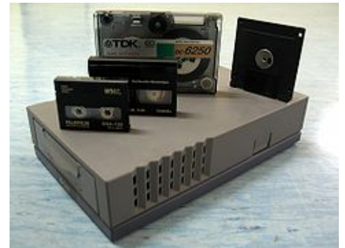
DDS tape drive with 4 types of magnetic data storage media on top, from right hand side: 3.5" floppy disk (1.44 MB), 310m QIC DC tape (250 MB, ~6 mm wide, 1020 ft length), 112m Data8 tape (5 GB, 8 mm, 367 ft), 150m DDS-4 tape (20 GB, 4 mm, 492 ft)
