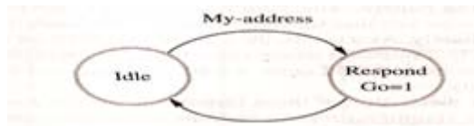
Fig 18 State diagram for the timing logic.
