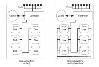
**Figure 2.5** In active cabling all hard disks are connected by just one I/O channel. In active/passive cabling all hard disks are additionally connected by a second I/O channel. If the primary I/O channel fails, the disk subsystem switches to the second I/O channel.
