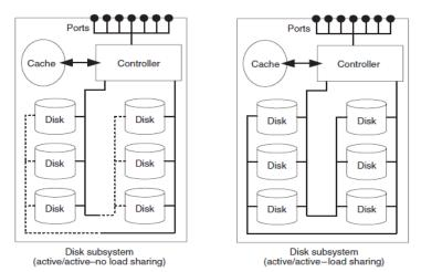
**Figure 2.6** Active/active cabling (no load sharing) uses both I/O channels at the same time. However, each disk is addressed via one I/O channel only, switching to the other channel in the event of a fault. In active/active cabling (load sharing) hard disks are addressed via both I/O channels.
