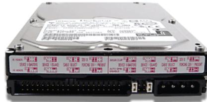
The drive type used most in consumer grade computers is the hardy ATA type drive (commonly called an IDE drive). The ATA standard dates back to 1986 and is based on a 16-bit parallel interface which has undergone many evolutions since its introduction to increase the speed and size of the drives that it can support. The latest standard is ATA-7 (first introduced in 2001 by the T13 Technical Committee (the group responsible for the ATA
