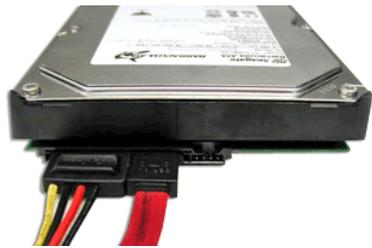
SATA drives are easy to distinguish from their ATA cousins by the different data and power connections found on the back of the drives. A side-by-side comparison of the two interfaces can be seen in this PDF from Maxtor, and the following covers many of the differences...
