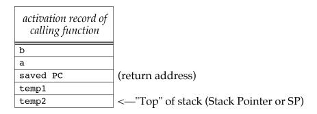
Given the arrangement of parameters and local variables in our protocol, we can think of an activation record as similar to 2 neighboring structs, one for the local variable block and another block for the parameter, with the saved return address in the middle. The sp is pointing to the base address of the local variable block, the return address follows, and the parameter block begins right after that.
