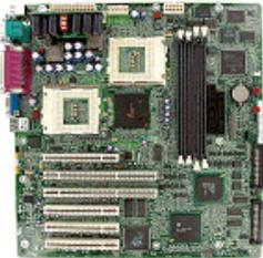
The Intel STL2 Dual Socket 370 Server Board is a good reference for comparing 32-bit and 64-bit PCI slots.
