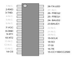
Figure 3. The diagram of RF Transreceiver pin configuration
