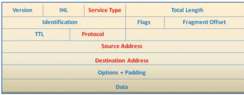
IP Packet Fields (Fields marked in red are prone to spoofing attack)
