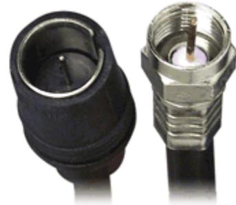
Those F connectors are a bear to screw in when you have to reach around behind a TV. First, you want to get that center conductor of the plug lined up and poked into the hole in the jack. Then, you need to carefully align the plug and push it against the jack as you turn the rotating part of the plug. Don't twist the cable, just the little nut on the plug. The trick to smooth threading of the plug onto the jack is to have it lined exactly up with no sideways pressure.
