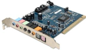
The basic computer sound system starts with a sound card, either a real pluggable card or one integrated into the motherboard. The traditional sound card has four stereo 3.5 millimeter jacks for inputs and outputs. One jack is a direct microphone input and one can drive a pair of speakers or headphones. Two other jacks are for Line In and Line Out. We will discuss these two a bit later. You can use the microphone and speaker jacks to hook up a headset for Internet VOIP phone calls or gaming.
