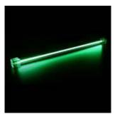
Want one more type of lighting that can be used to mod a case? Good. EL, or Electro Luminescent lighting, can be found in a variety of products, and it is distinguished by its even glow, long life, and low power consumption. Products such as keyboards and case badges are just two products that take advantage of the cool lighting effect provided by this high tech, thin material.
