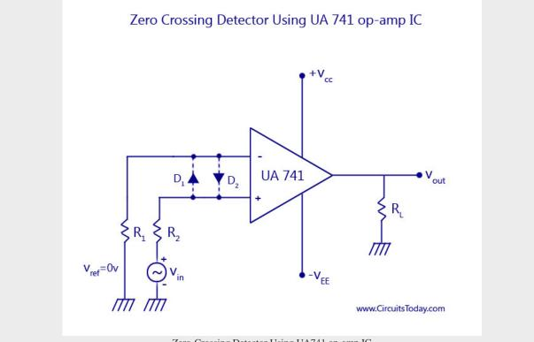
Zero-Crossing Detector Using UA741 op-amp IC
