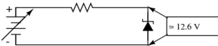
Zener diode regulator circuit, Zener voltage = 12.6V).
