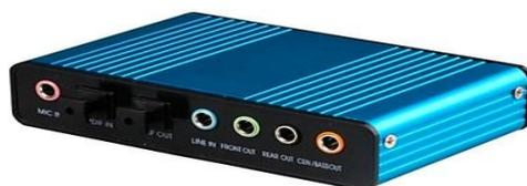
Lots of people seem to be making interfaces based around the C-Media CM6206 (and cousins). They are cheap (about £7), and full-featured: 5.1 analogue outputs, stereo inputs, and optical input and output. Sadly though, the frequency response isn't great. I measured the -3dB points at about 42Hz and 19.6kHz (44.1kHz sampling rate).
