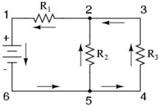
In this circuit, we have two loops for electrons to flow through: one from 6 to 5 to 2 to 1 and back to 6 again, and another from 6 to 5 to 4 to 3 to 2 to 1 and back to 6 again. Notice how both current paths go through  $R_1$  (from point 2 to point 1). In this configuration, we'd say that  $R_2$  and  $R_3$  are in parallel with each other, while  $R_1$  is in series with the parallel combination of  $R_2$  and  $R_3$ .
