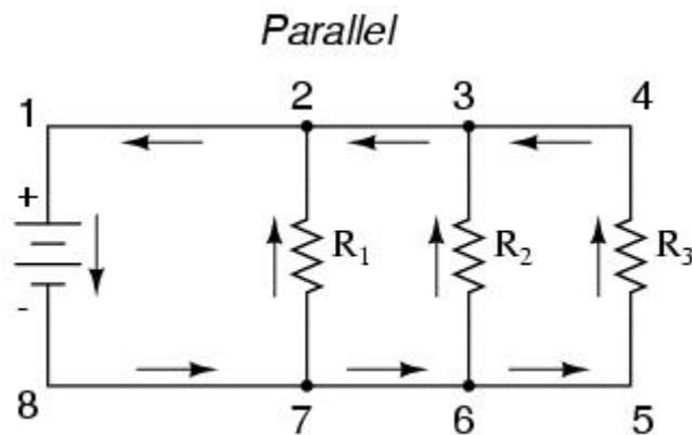
Again, we have three resistors, but this time they form more than one continuous path for electrons to flow. There's one path from 8 to 7 to 2 to 1 and back to 8 again. There's another from 8 to 7 to 6 to 3 to 2 to 1 and back to 8 again. And then there's a third path from 8 to 7 to 6 to 5 to 4 to 3 to 2 to 1 and back to 8 again. Each individual path (through  $R_1$ ,  $R_2$ , and  $R_3$ ) is called a branch.
