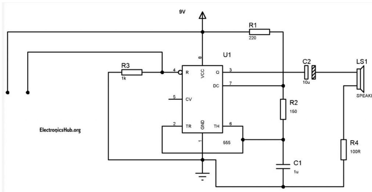
Circuit Diagram of Water Level Alarm using 555 Timer – [ElectronicsHub.Org](http://ElectronicsHub.Org)
