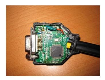
Cracking open the shell wasn't trivial, since the whole thing is filled with hot glue. However a careful application of a hair drier and various sizes of flat screwdrivers did the trick. It still works (minus one SMD capacitor I managed to tear off), however I pretty much demolished the case.
