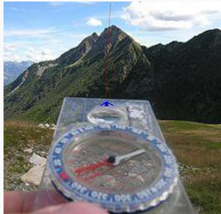
When the needle is aligned with and superimposed over the outlined orienting arrow on the bottom of the capsule, the degree figure on the compass ring at the direction-of-travel (DOT) indicator gives the magnetic bearing to the target (mountain).
