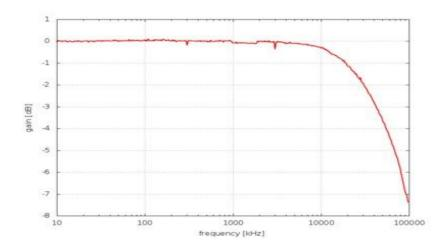
This shows that the -3 dB frequency is surprisingly high, at around 42 MHz. This is not something I expected - I thought the roll-off would start not much beyond the Nyquist frequency. Also, the specified sampling time of 0.11  $\mu$ s gave me the impression that the analog bandwidth would be below 10 MHz. Actually, above 10 MHz the attenuation I saw might as well come from stray capacitances in the circuit and not from the converter itself.
