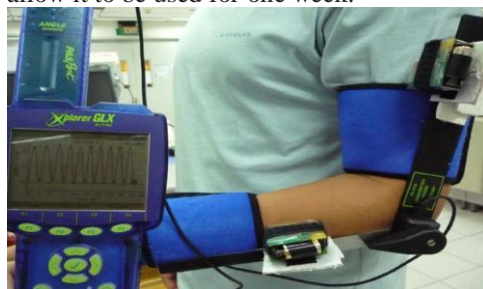
Fig. 15. Angle between the forearm and the upper limb obtained using the sensor nodes and a goniometer at different speeds.
