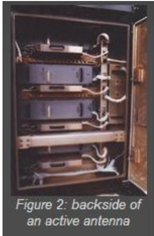
Figure 2: backside of an active antenna
