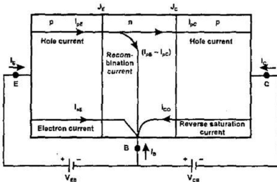
*Fig.2.9. Transistor current components*
