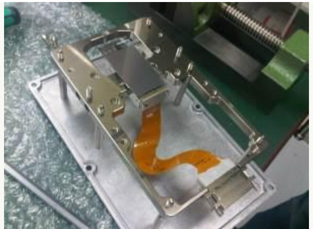
One of the expensive CCD test chips. It has 512 \times 1024 pixels. Each pixel is 50 micrometers wide – quite large, so that only 3000 photons are needed to generate a signal.
