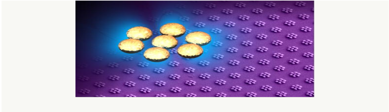
Gold heptamer structures show strong Fano resonances. The gold nanoparticles are only about 150 nanometers in diameter. (c) Sven Hein, Na Liu, Harald Giessen, University of Stuttgart, Germany.
