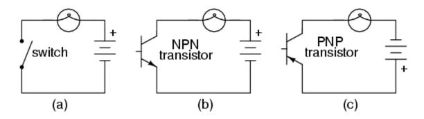
(a) mechanical switch, (b) NPN transistor switch, (c) PNP transistor switch. A PNP transistor could also have been chosen for the job. Its application is shown in Figure <u>above(c)</u>.
