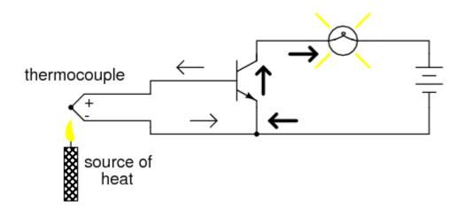
A single thermocouple provides 10s of mV. Many in series could produce in excess of the 0.7 V transistor  $V_{BE}$  to cause base current flow and consequent collector current to the lamp.
