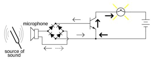
Amplified microphone signal is rectified to DC bias the base of the transistor providing a larger collector current.
