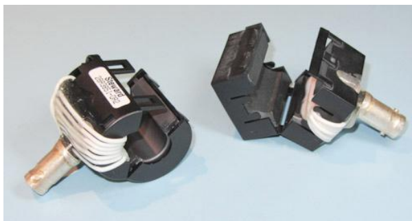
Figure 5. Examples of DIY current probes based on clamp-on ferrite chokes. I used a couple sample Steward (now a unit of Laird Technologies) chokes – a round one (model 28A3851-0A2) and a square one (model 28A2024-0A2). They each had 7 turns of Teflon-insulated wire wound around one-half and glued down on the inside to hold the windings. I later epoxied a PC board-style BNC connector to the outside, making sure there was enough epoxy to hold the outer turns together. Type 28 material was used, which is useful from 10 to 1000 MHz.
