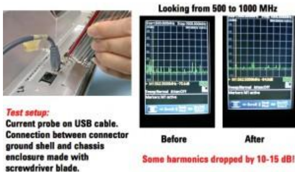
Figure 11. Cables should be tested individually. Here, I have a current probe clamped around the cable under test and am monitoring the harmonics with a simple hand-held spectrum analyzer. As I ground the connector shell to the chassis with the Swiss Army screwdriver blade, the harmonics were reduced 10-15 dB!
